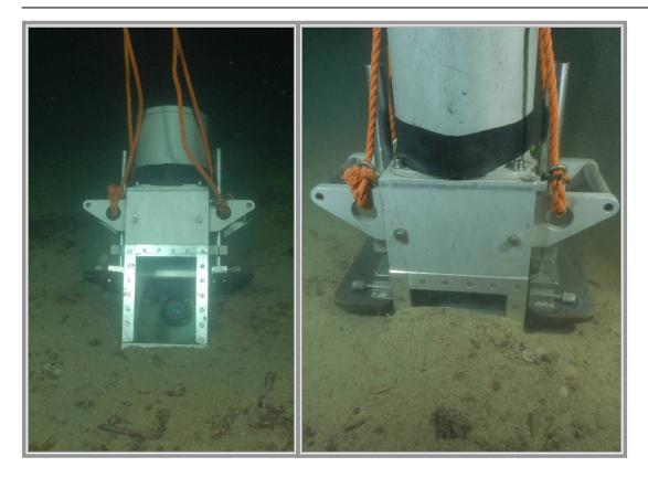
Figure 2.1. Diver operated Sediment Profile Imaging camera. The left-hand image gives a view of the camera at the sediment surface. The right-hand image shows the SPI camera when inserted into the sediment.
